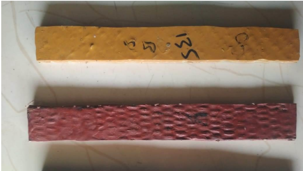
Fig.8 Sample of Flexural Test specimens
