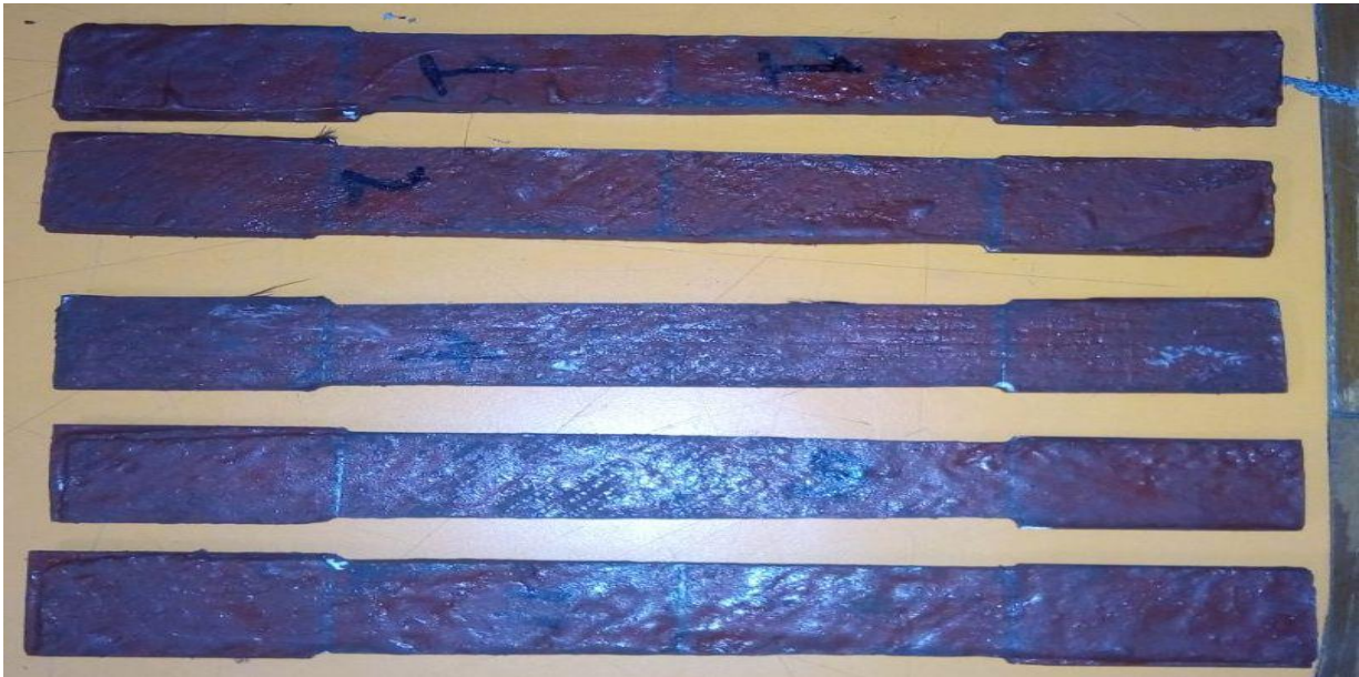
Fig.4 Sample of Tensile Test specimens.
