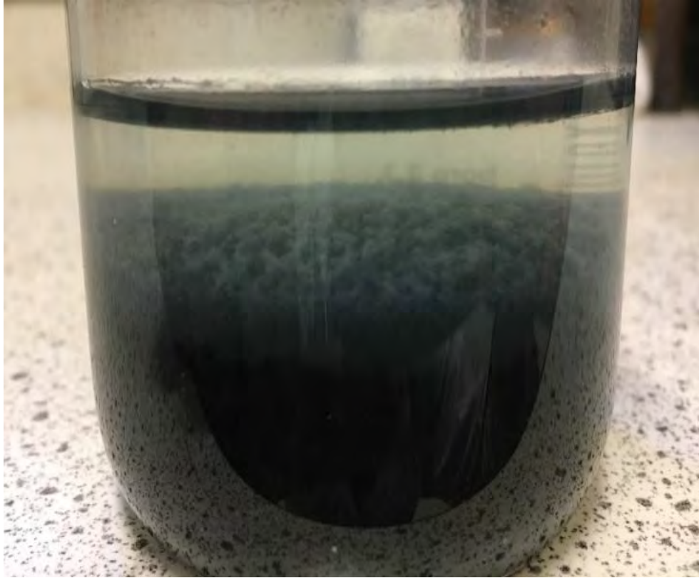
Figure 3.1. Laboratory solvent impregnation onto the AC surface
