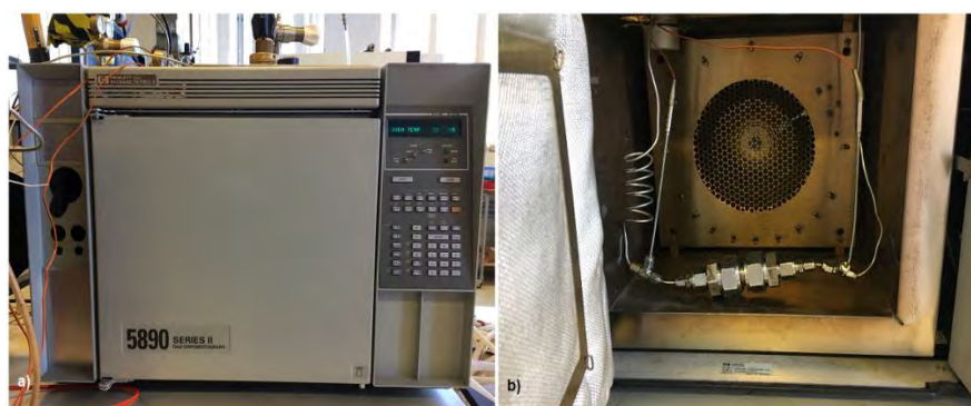
Figure 3.5. A) Oven used to heat the reactor and provide a stable temperature for PSA tests, and B) FBR inside the oven with the two thermocouples inserted at the gas flow inlet and outlet
