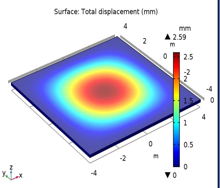
Results of applying a pressure Results of applying a of 500N/m<sup>2</sup>
