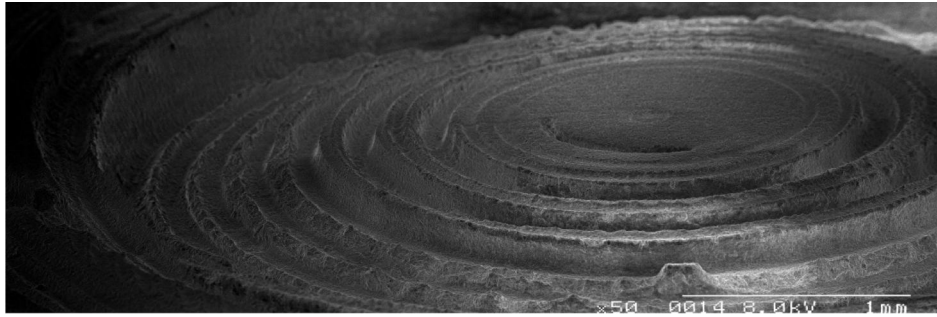
Figure 3.5: Scanning electron micrograph of a prototype Shapal Hi-M Soft Fresnel lens.
