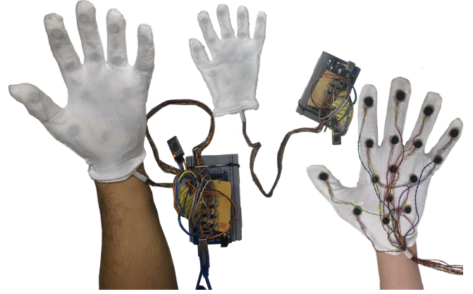
FIGURE 3. Haptic glove (left module shown) in its final and first iteration with its electronics and motors exposed in the latter.
