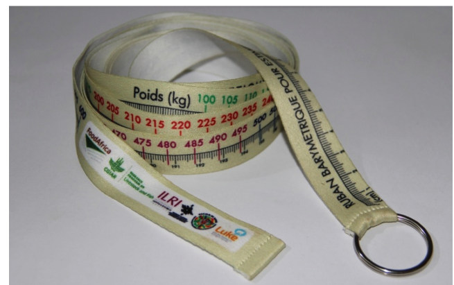
Figure 1. Tape for measuring heart girth of animals for the prediction of body weight.
