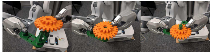
Fig. 7: The execution of a neural network policy for inserting the gear on the peg.
