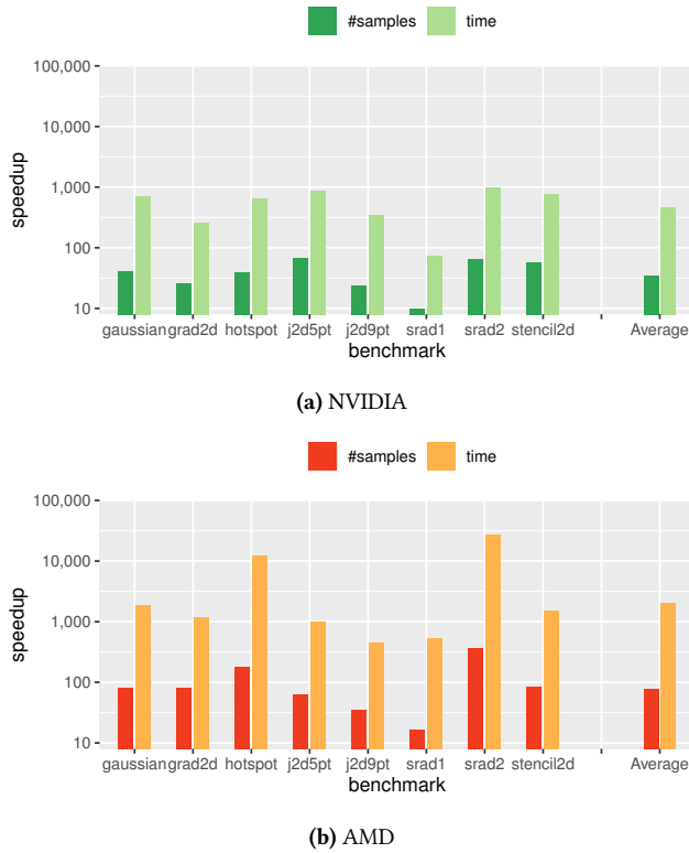
Figure 6. Reduction in the number of samples and corresponding time required to explore to reach at least 90% of the available performance (average = geometric mean).
