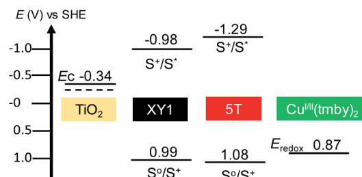
Fig. 2 Energy diagram of the dyes used in this study, in comparison with the TiO 2 anode and Cu I/II (tmby) 2 electrolyte. All state levels are described in volts. The values were taken from the literature. 38,41,48
