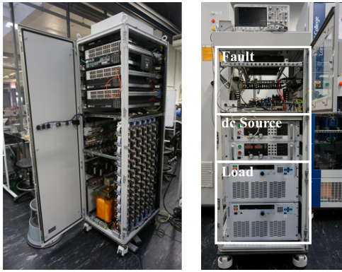
Fig. 12. Experimental set-up of converter, fault and dc source and load.
