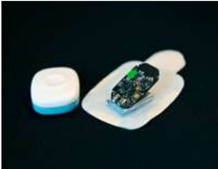
Figure 1. The Respeck sensor worn as a plaster on the chest.
