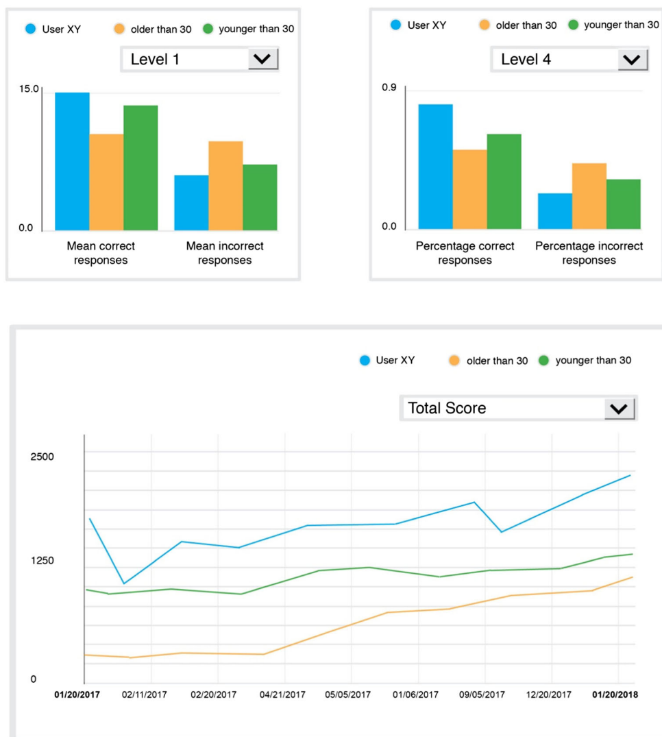
Fig. 2 Example of a typical visualization of test results generated by the mongoDB-based visualization feature of the COSMOS web platform. The generated graphical representations are partially configurable and allow the user to customize which data is displayed. Any data fed into the mongoDB can be visualized in either bar charts, pie charts, or progress charts. Database schema of the game Frog Life
