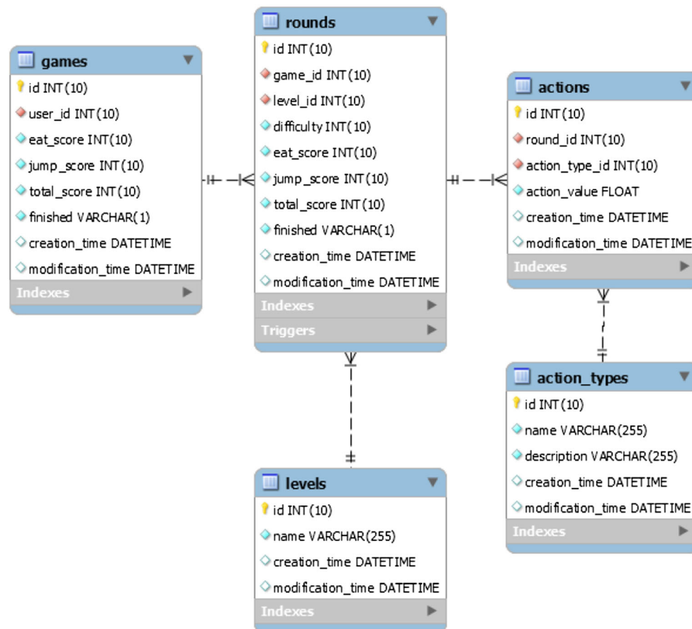
Fig. 3 The SQL database schema for Frog Life. The games-table records all the games (numbered incrementally starting from 1) a given user (user_id defined by the UIC) has played, along with the scores s/he achieved and the timestamp the game was started (creation_time) and finished (modification_time). The finished field contains the info whether the game was normally finished or prematurely terminated. All lines between the tables are dotted, since the UIC serves as foreign key for all other tables. The rounds-table contains information about every single round played as indicated by the “one to one or many” relationship (since many rounds per game are possible). A round starts either directly at the beginning of the game or after the player escaped an upcoming predator
