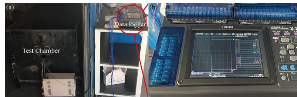
257 Fig. 7. Devices for thermal runaway experiment
