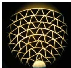
Figure 5: The rotary wheel is assumed to be composed of corrugated channels, similar to those shown in the figure (image from Mohammadi, 2017)
