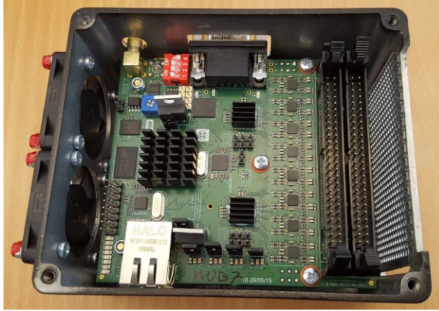
Fig.5. A custom digitization node with a central FPGA (A), two octal ADC packages (B), main clocking phase locked-loop (PLL) (C), Ethernet communications (D) and initial analog filtering (E). Also included are i) SDRAM and FLASH memories, ii) PROM for FPGA configuration and bootloader, iii) a 3-axis accelerometer and iv) a 12-bit temperature sensor. Below the main PCB is a secondary power regulation PCB delivering \pm 5 V 1 A for up to 16 photodiode preamplifiers.
