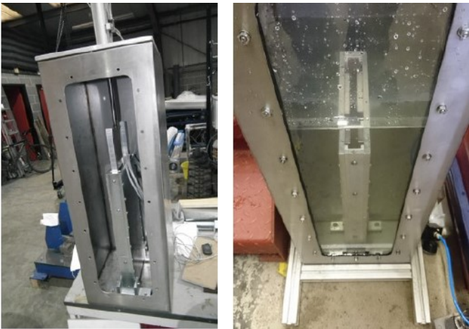
Figure 16. Linear test rig for testing thermal performance
