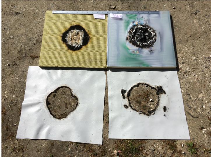
Figure 7 - Two of the mass loss experiments were carried out with a 0.60 m by 0.60 m section of a mitigation solution with a mitigation layer of either mineral wool (upper left) or PIR insulation (upper right) and the roofing membranes (front). An area with the width of approximately 1/3 of the total width was affected by the wood crib fire in all four experiments, defining the domain/distance where the heat from the wood crib can ignite the surrounding construction materials.
