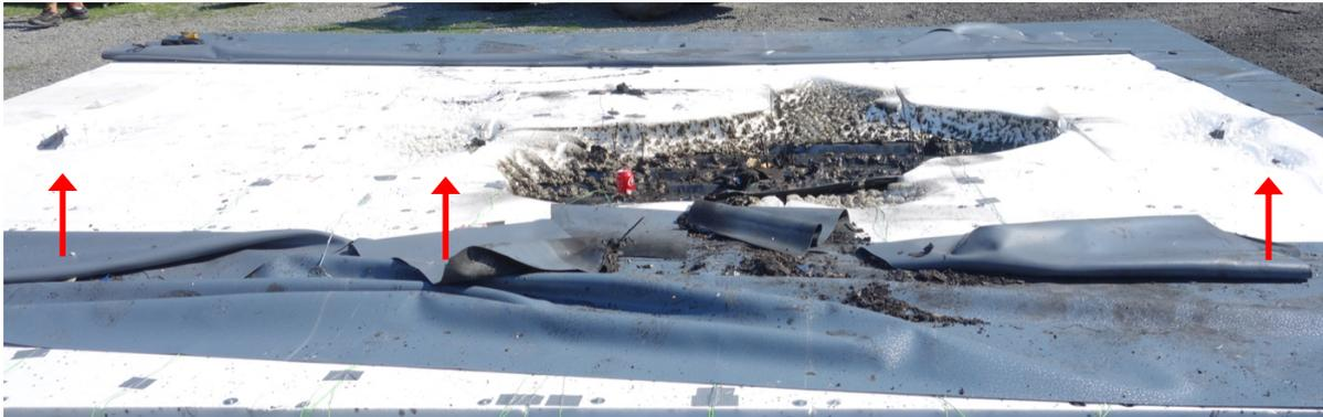
a) From experiment T3 (PIR insulation). The damaged area was limited due to extinguishment by fire fighters. Notice; 1) the sooty sides of the EPS insulation and the carbonised area in the centre of the hole. 2) The melted areas above the three red arrows. The observed smoke production and the recorded temperatures also support the postulation that the EPS ignited.
