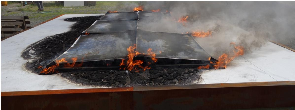
Figure 10 - Experiment T3. The whole area underneath the PV array was affected by the fire. Contrary to the picture, the dominant wind direction was from the right towards the left side of the picture as seen in Fig. 10 a.
