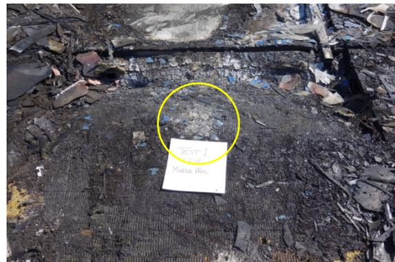
Figure 13 – Experiment T4. Part of mock-up cleared from leftovers and PV panel. Approximate width of the picture at centre: 1.2 m. Yellow circle: Point of ignition without penetration of the mineral wool.
