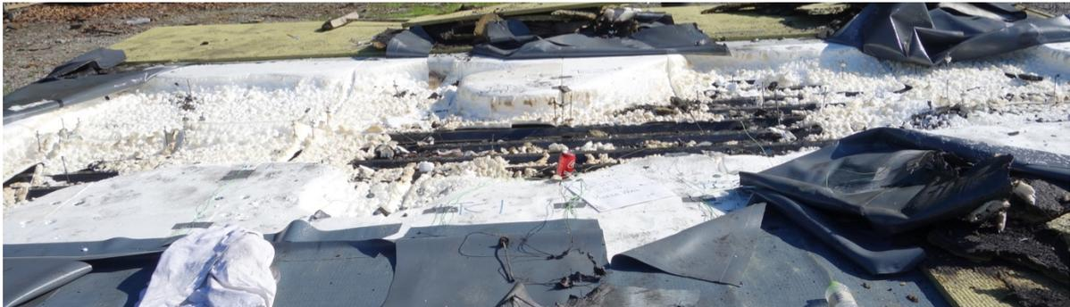
b) From T4 (mineral wool). The absence of soot on the EPS insulation, combined with the lack of smoke observations and the low recorded temperatures, suggests that no ignition occurred, and the damage of the EPS only happened due to the conductive heat transfer through the mineral wool.
