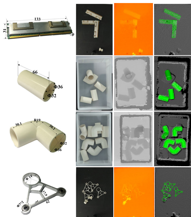
FIGURE 11. Multiple object detection, where the first column is the RGB image ( computer-memory-card , two-way-joint , corner-joint and aluminum-motor-support-ring ), the second column is depth image (the first and last depth are highlighted with pseudo color), and the last column is the target with the green pose mask produced using our algorithm.
