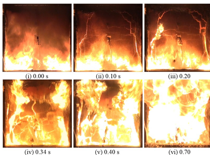
(a) Breakage and fall out
