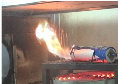
(c) After 22s carbon dioxide was applied
