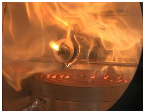
(b) 2 s after ignition, both cathode and anode caught on fire
