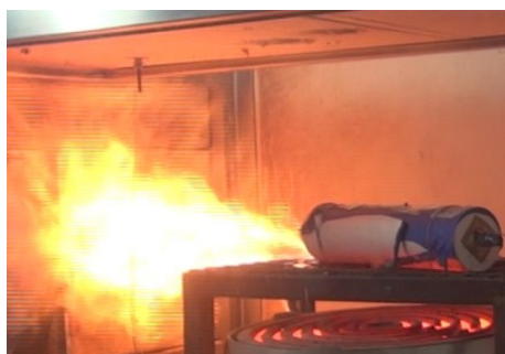
(a) The jet fire was formed
