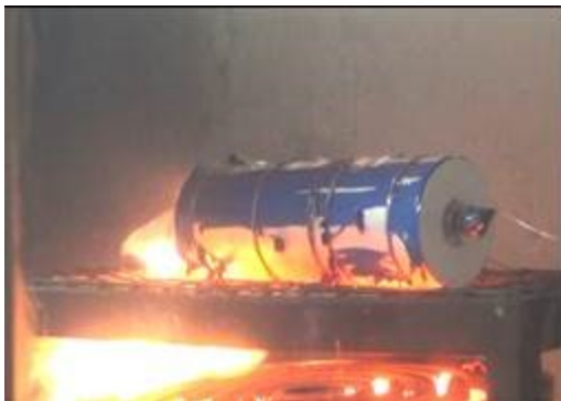
(a) The dropped electrolyte was ignited
