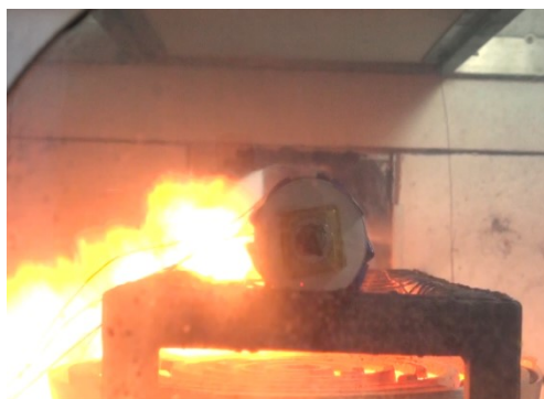
(a) 1079 s after oven heated the battery, the dropped electrolyte was ignited
