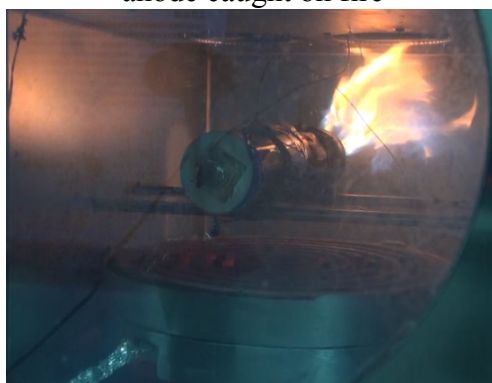
(d) The fire was under control, 24 s after ignition the fire was put out
