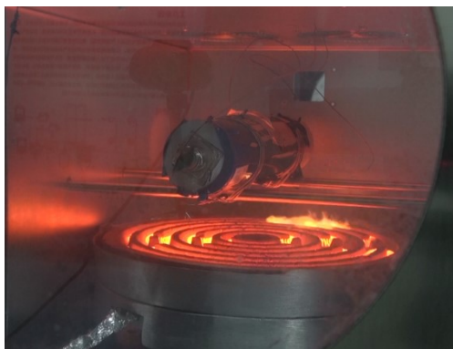
(a) 859 s after oven heated the battery, the dropped electrolyte was ignited
