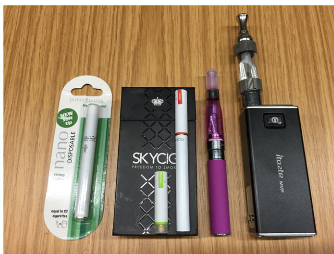
Figure 1 E-cigarette props used in interviews. From left to right: disposable cigalike, reusable cigalike with interchangeable flavours (packet contents on exterior), vapouriser, box mod.
