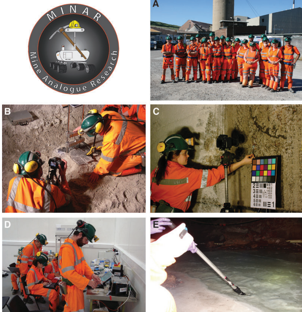
FIG. 9. The MINAR program uses the Boulby Mine in the United Kingdom as a deep subsurface analog site. (A) The MINAR 4 team (2016) from the European Science Foundation, the Spanish Centre for Astrobiology, the University of Leicester, the University of Edinburgh, and Universidad Autonoma de Madrid. (B) Testing a robotic geologist's hammer (SPLIT) (University of Leicester). (C) Testing of the Panoramic Emulator Camera (PanCam) (University of Aberystwyth). (D) Testing of SOLID (Signs of Life Detector) in the underground astrobiology laboratory (BISAL) (Spanish Centre for Astrobiology). (E) Collecting anoxic sediments to characterize the microbial communities in the framework of the EU project MASE.
