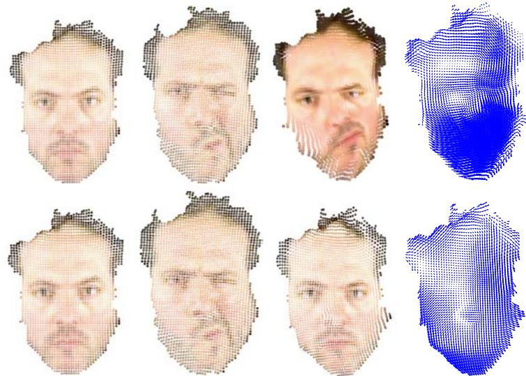
Figure 22: Real data registration, large deformation. The top row is CCPD, and the second CPD. From left to right, original deformation, target shape, registered shape, and data flow
