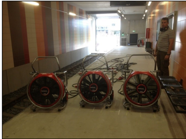
Figure 7 Three fans placed on the platform in the Frankfurt subway building. The fans are positioned with reference to the centre line of the stairs. From right to left: -25cm, +67cm and +150cm. The stairs are behind the photographer. The fan on the right in the picture is addressed as 'left' in the text and vice versa.
