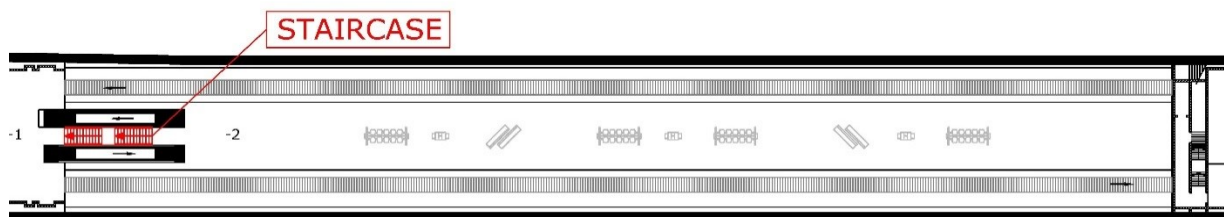
Figure 12 Floor plan of a subway station with two tracks and one, central platform. The staircase is on the left-side of the floorplan. This floor plan is shown for illustrative purposes only.
