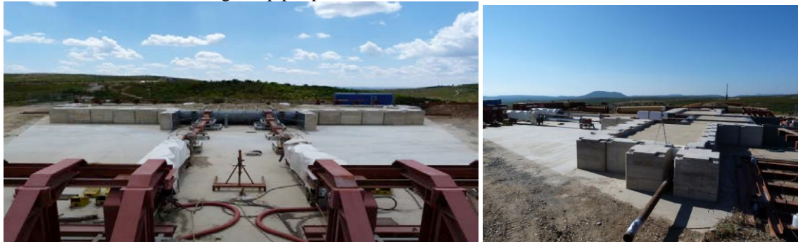
Figure 29. Views of experimental setup of "landslide/fault" tests; actuators and soil boxes.
