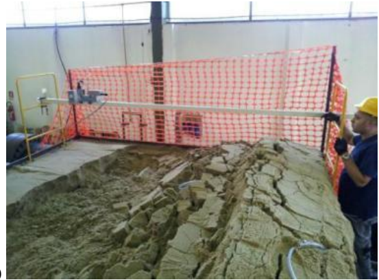
Figure 16. Transverse soil-pipe interaction; (a) test setup before backfilling; (b) soil surface after the test.
