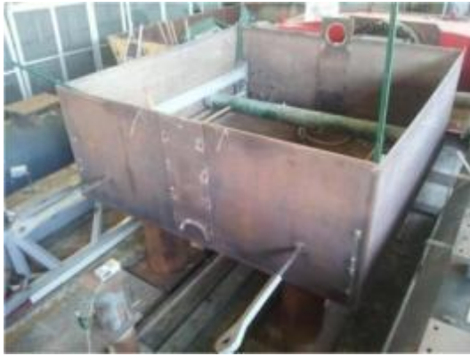
Figure 16. Transverse soil-pipe interaction; (a) test setup before backfilling; (b) soil surface after the test.
