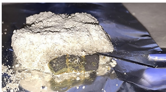
Fig. 2. Post-extraction picture of the corroded uncoated NdFeB magnets still encased in the bentonite matrix. Tip of the scalpel used as a reference.
