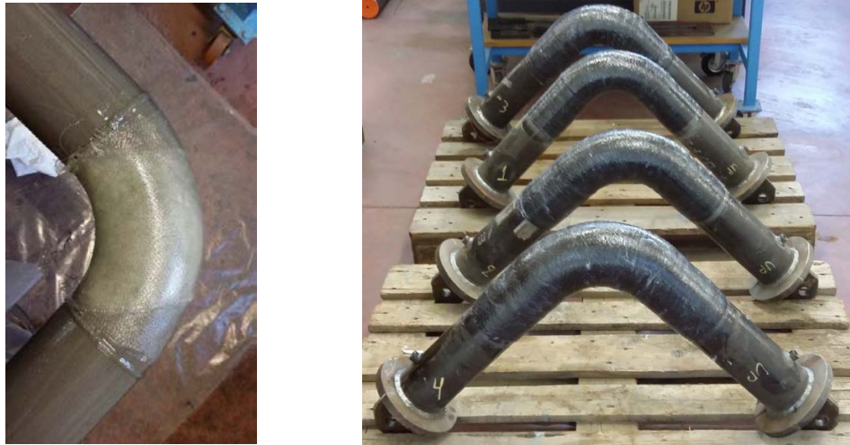
Fig. 11: Repair of cracked non-reinforced specimens, with CFRP/GFRP wrapping.
