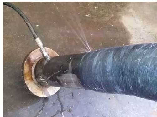
Fig. 12: Burst and loss of containment in CFRP repaired specimens due to burst (specimen 4).
