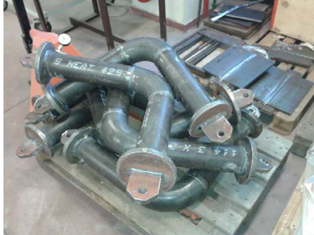
Fig. 1: Steel elbow specimens.
