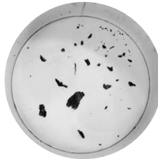
Fig. 3. Standardized photograph of the inside of a typical aluminum firebrand collection can (diameter: 22 cm) with firebrands.
