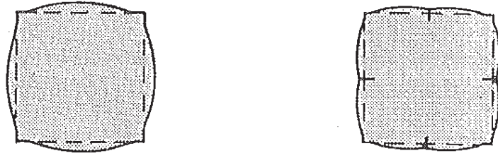
(a) Local buckling of unstiffened CFST section (b) Local buckling of stiffened CFST section
