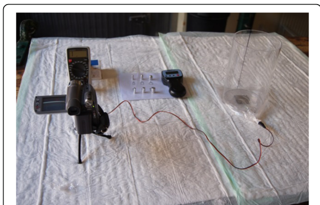
Fig. 3 Measurement set-up for the post mortem specimens. On the left there is multimeter and the video camera, in the middle is the algometer with the tips used and on the right is the pressure sensor below the plexiglass cylinder later containing the tissue section
