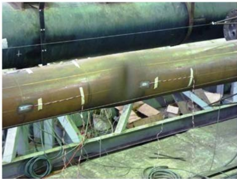
Figure 5. Axial compression tests: (a) short specimen AS1 with local buckling near its end (top); (b) and (c) long specimen AL1 with global buckling (bottom left) followed by local buckling (bottom right).
