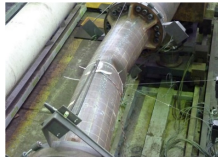
Figure 7. Buckled specimens under combined loading tests; specimen (a) BS-13 and (b) BS-75.
