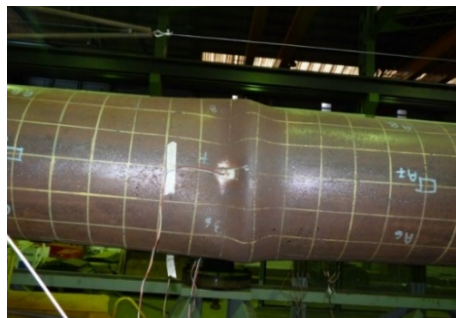
Figure 7. Buckled specimens under combined loading tests; specimen (a) BS-13 and (b) BS-75.
