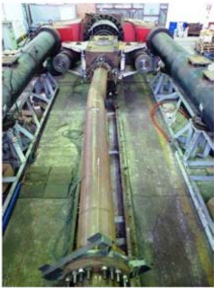
Figure 5. Axial compression tests: (a) short specimen AS1 with local buckling near its end (top); (b) and (c) long specimen AL1 with global buckling (bottom left) followed by local buckling (bottom right).
