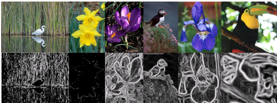
Fig. 7. Birds and Flowers Original (1 st row) and edge images (2 nd row). 1 st column shows for a Birds image the Edge Image after applying the compass operator with r=0.75 . It can be observed that there are more edges from the background than from the bird. 2 nd column shows for a Flower dataset image the resulting image after apply r=0.75 too. There are not enough edges to describe the object. Columns 3 to 6 show samples from both datasets with r=15 applied. The edge objects are blurred.
