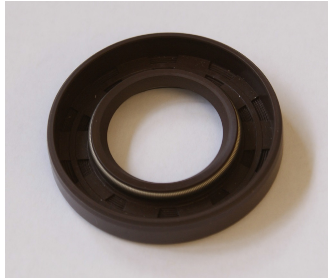
Fig. 19. Viton lip seal with visible stainless steel lip spring.
