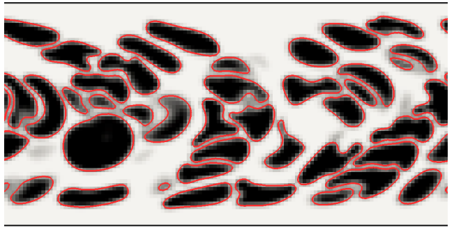
Fig. 2 Indicator field I(\mathbf{x}) for distinguishing between interior and exterior fluid sites. A two-dimensional cross-section of a three-dimensional RBC suspension in a tube is shown. Red lines denote the Lagrangian membranes. The grey-scale lattice-like portion of the figure reflects I(\mathbf{x}) on the same cross-section. Black denotes the interior, white the exterior.
