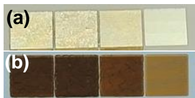
Figure 1. Photos of the laser modified areas of the sample. From left to right areas #1 - #4. The sizes of the squares are 2.4 \times 2.4 \text{mm}^2 . Images (a) and (b) were taken with different illumination.
