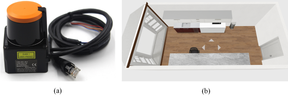
Fig. 7. (a) UST-10LX LIDAR, (b) Kitchen scenario
