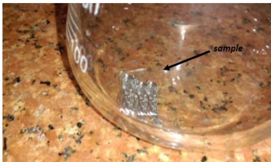
Fig.1. The fixation of sample with epoxy resin.
