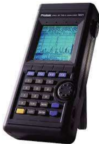
Figure 3. Picture of MIT model 3201 RF field strength analyzer tuned to 1.420405 GHz.
