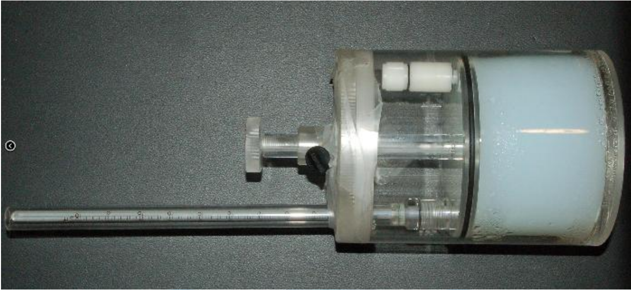
Fig. 1: The phantom realized by the Medical Physics Unit of the AOUC of Florence, Italy. It is a plexiglass cylinder, filled with an aqueous solution of Agarose (1.2% weight fraction) with a thermometer in close contact with the solution.
