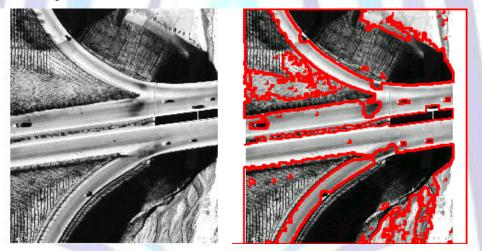
Figure3(a) original image (b)extracted road vector
