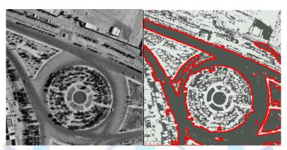
Figure2(a) original image (b)extracted road vector
