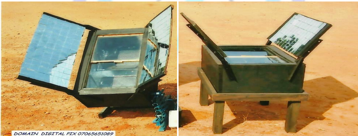
Figure 1(c):Both box cookers showing sub-sized mirror reflectors to boost input power, and the double sliding glass cover for the cooking chambers with perfect insulation.
