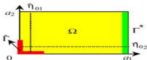
Fig. 6: Rectangular domain \Omega , region \Gamma^* and location \bar{\Gamma} of boundary zone sensor.
