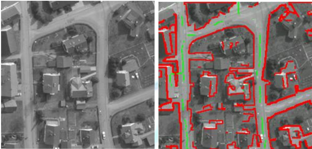
Fig 2: Extraction of straight line segments. (a) Original SAR image and (b) extracted straight line segments in the preprocessed SAR image.
