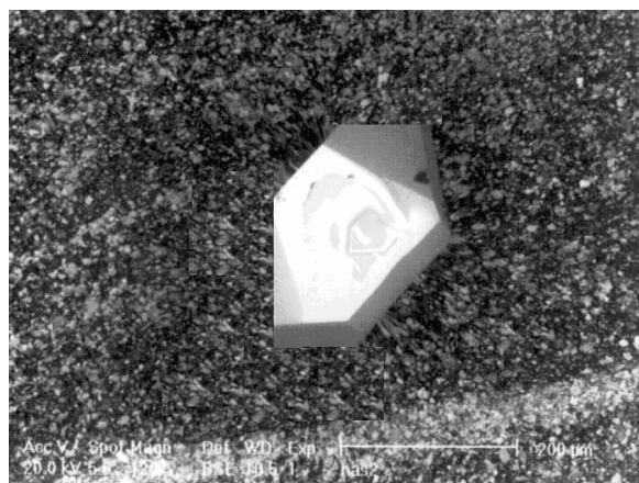
Figure 1: Photograph of single crystal of \text{RbBi}(\text{PO}_3)_4 grown by the flux method
