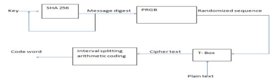
Fig2 shows proposed scheme of T box
