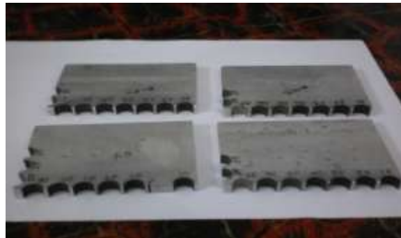
Fig.5b. AA6063/SiC Plate after machining
