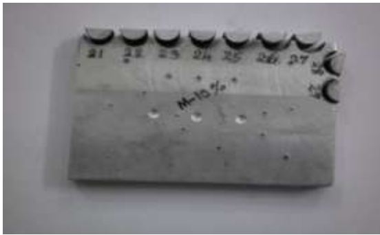
Fig.5a. AA6063/SiC Plate shows circular contour
