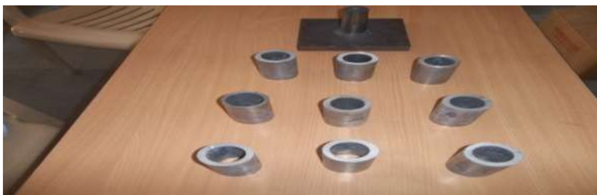
Fig.2 Squeeze casted samples
