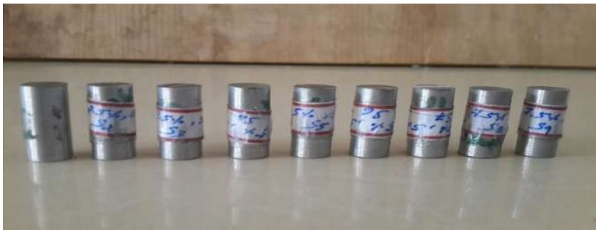
Fig 3.Specimens used for wear test
