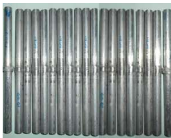
Fig 2: After welding (AA6061 and AA201)
