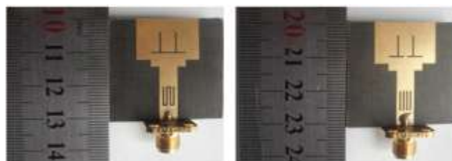
Fig. 6 Photograph of triple band reconfigurable filter
