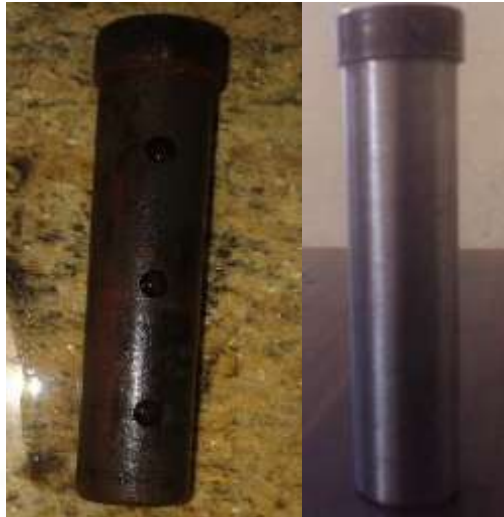
Fig 3: Work piece before and after quenching
